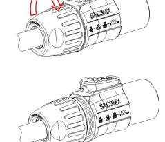
Note: This product is equipped with two sizes of waterproof rubber rings on the strain relief as standard. They are applicable to different cable diameters and can be replaced by the customers according to the diameter of the cable used, as shown in the picture.
