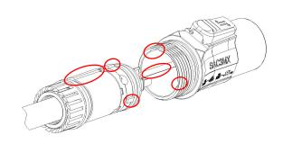
(5) After the assembly of the strain relief, inner core component and housing, tighten the bushing in a clockwise direction with a torque of 2.0 Nm.
